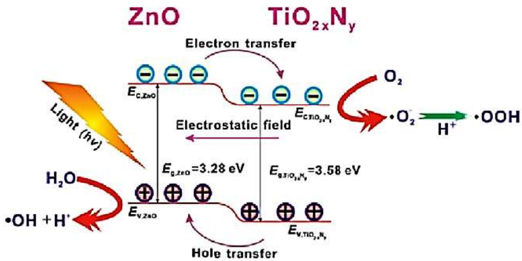
Figure 15: Photogenerated charge separation mechanism of ZnO coupled with \text{TiO}_{2x}\text{N}_y [259].
